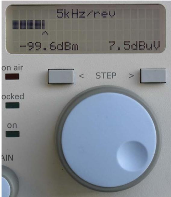
The frequency is set by the large rotary knob. The resolution of the encoder is 1000 pulses per revolution. The frequency rate per revolution may be set by the keys STEP < and > resulting in a range of 500Hz and 100kHz. A new selected value is indicated in each case on the top of the small display for 5 sec. For very fast rotation, the frequency change increased progressively and at a very slow rotation it is gradually decreased. In between is a large linear range.
