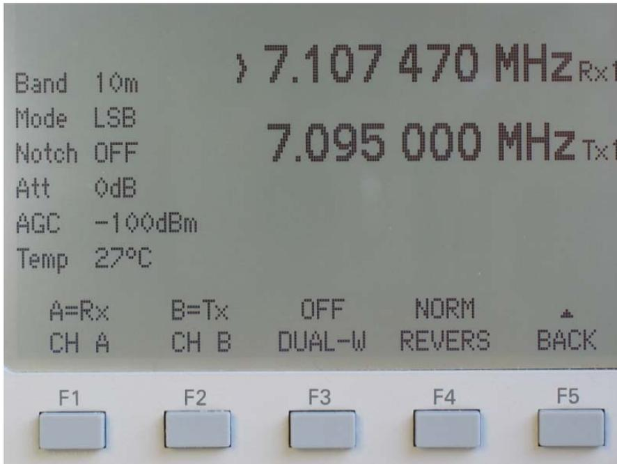
The frequencies of A and B are each presented on the display with large figures. Basically, the channel A is only used for reception (Rx1), while the channel B is dedicated to receive and transmit (Tx1). The currently selected channel is marked with an arrow. Its frequency can be changed with the frequency tuning knob.
